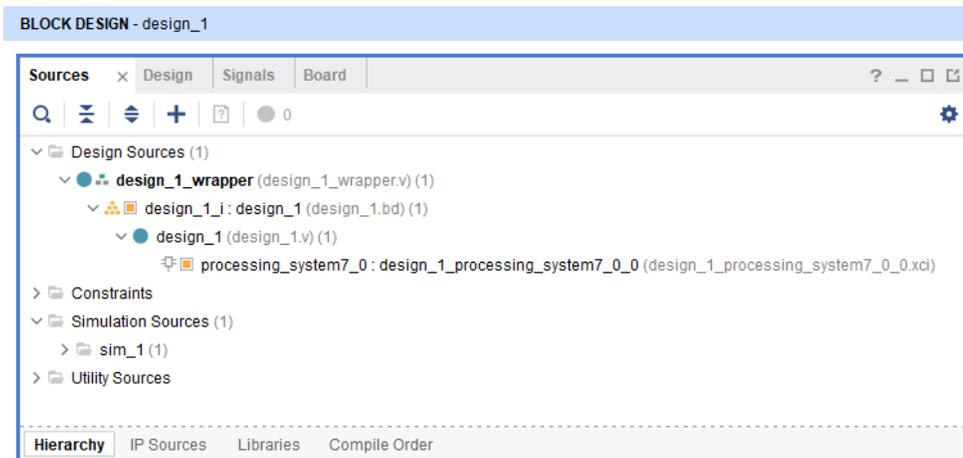
**Figure 8 – System\_wrapper.vhd Generated**
